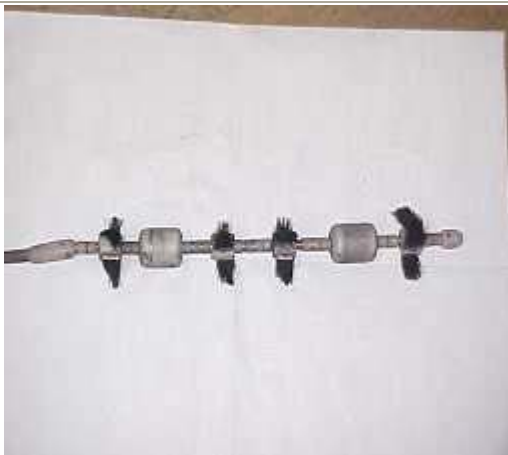
These pictures show the Eagle 2000 Plus Multichannel Probe . These probes are flexible; this allows the bends to be tested with full detection/quantification capabilities.
