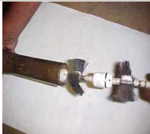
These pictures show the Eagle 2000 Plus Multichannel Probe . These probes are flexible; this allows the bends to be tested with full detection/quantification capabilities.
